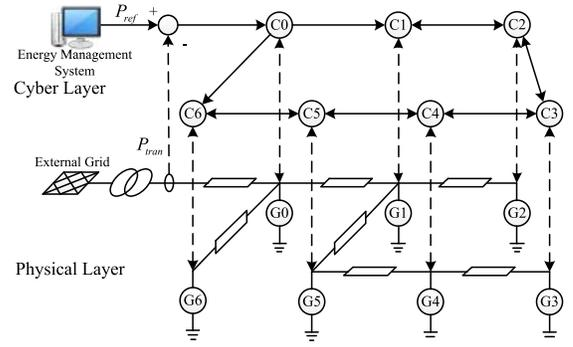
Fig. 1. Diagram of the cooperative control of DGs. Solid arrow denotes communication within the cyber layer and dash arrow denotes communication between the physical and cyber layers.
