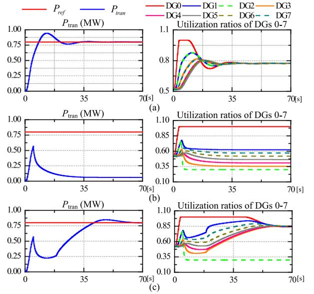
Fig. 6. Responses of the non-resilient/resilient cooperative control system with/without replay attack on DG 2: (a) Non-resilient cooperative control without replay attack, (b) Non-resilient cooperative control and (c) resilient cooperative control when DG 2 is under replay attack.
