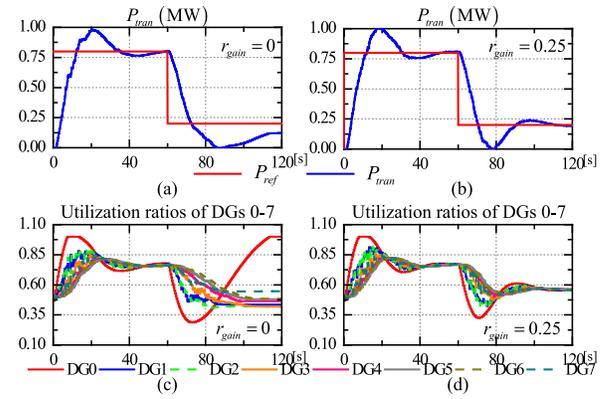
Fig. 8. Response of the VPP with the attack-resilient cooperative control ( $r_{\text{gain}} = 0$  and 0.25) in the presence of packet loss: (a-b) Power flow across the transmission line (MW); (c-d) Utilization ratios of the DGs.
