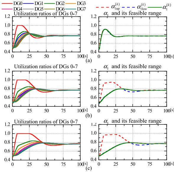
Fig. 7. Response of the VPP when DG 1 is under stealthy attack: (a)  $\eta = 0.2$ ; (b)  $\eta = 0.1$ ; (c)  $\eta = 0.05$
