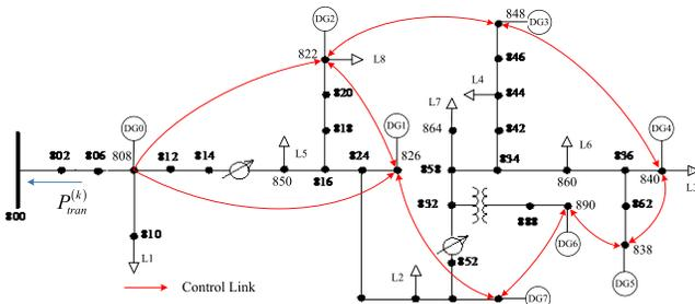
Fig. 5. Diagram of the IEEE 34-bus test feeder.
