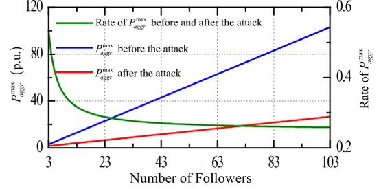
Fig. 3.  $P_{aggr}^{\max}$  before and after cyber-attack on DG 1 ( $\alpha_1^{(k)} \equiv 0$ ) with different NCS size from  $n = 3$  to  $n = 103$ .
