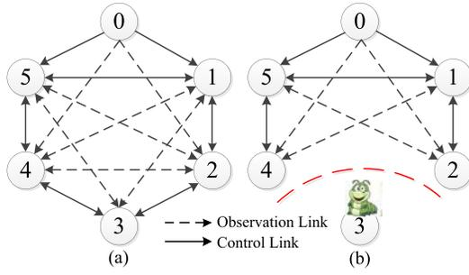
Fig. 4. Diagrams of the communication network with control and observation links (an observation link is denoted as a solid arrow if it coincides with a control link): (a) A connected communication network; (b) The network after DG 3 is isolated due to cyber-attack.
