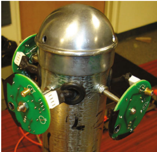
Fig. 5 Optical antenna with transceivers and SFH 4881 is replaced on to transceivers
