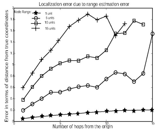
(c) Absolute error in terms of distance from correct coordinates due to an estimation error in range.
