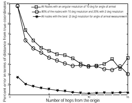
(b) Absolute error in terms of (percent) distance from correct coordinates due to an estimation error in orientation.
