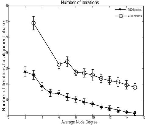
(a) Number of iterations needed to localize as a function of average node degree.
