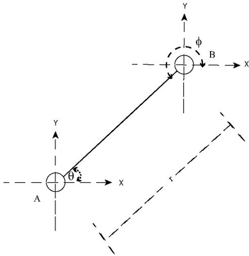
Fig. 1. Illustration of the principle of an FSO based location system.
