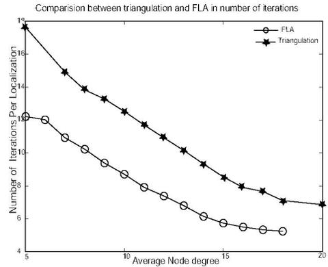
(a) Comparison of the number of iterations for localization for FLA and triangulation.
