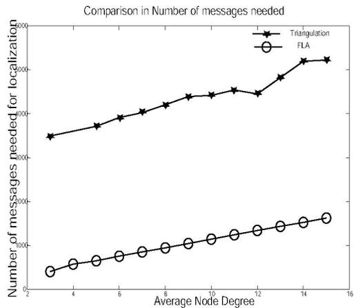
(b) Comparison between FLA and triangulation in terms of the number of control messages exchanged for localization.
