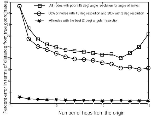
(a) Absolute error in terms of (percent) distance from correct coordinates due to an estimation error in orientation because of coarse angular resolution.
