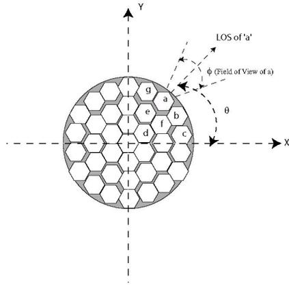
Fig. 2. FSO antenna for localization.
