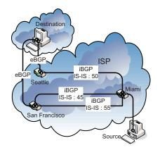
Figure 1. Example of Hot Potato Routing
