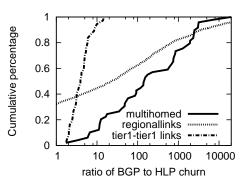
Figure 7: Churn: Comparing the churn reduction factor of HLP for different types of inter-AS link events.
