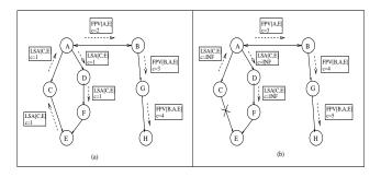
Figure 2: Basic HLP route propagation: Link failure example
