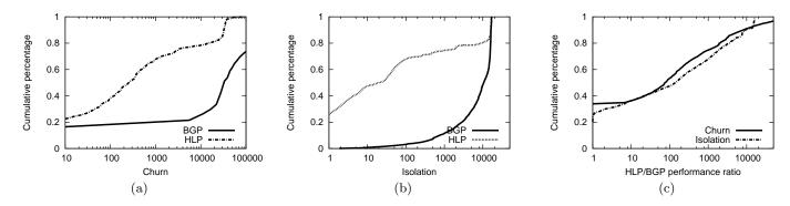
Figure 6: (a) Churn: CDF of the number of route updates generated by a single event in HLP and BGP. (b) Isolation: CDF of the region of visibility (measured in number of AS's) of the effects of a single routing event in HLP and BGP. (c) CDF of the churn improvement ratio and isolation ratio of HLP in comparison to BGP.
