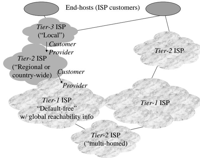
Figure 3: A more accurate picture of the wide-area Internet routing infrastructure, with various types of ISP’s defined by their respective reach. *Tier-1* ISP’s have “default-free” routing tables (i.e., they don’t have any default routes), and typically have global reachability information. There are a handful of these today (about five or so).
