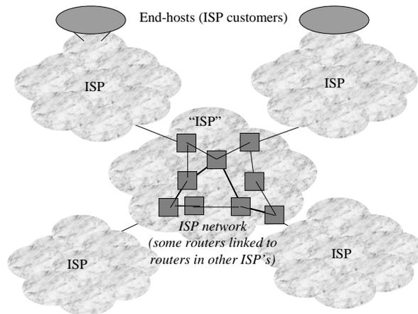
Figure 2: The Internet is actually composed of many competing Internet Service Providers (ISP's) that cooperate to provide global connectivity. This picture suggests that all ISP's are "equal," which isn't actually true.
