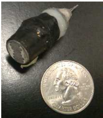
Fig. 12.3. Photo of the photoresistor to be used, which has already been waterproofed..
