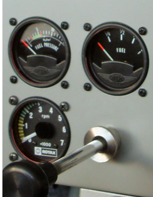
Figure 2-11: This is a close up of the fuel pressure gauge, the fuel gauge, and the tachometer in a real GoBosh (left to right top to bottom). Photo by Robert Gysi.
