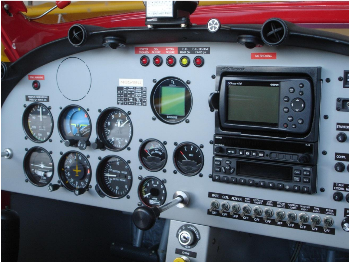
Figure 3-2. Gauges, switches and lights to be implemented. The “Six-pack” gauges are the cluster of six large gauges to the left of the picture. Photo by Robert Gysi.
