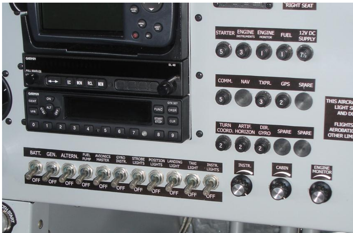
Figure 3-58. Switches and knobs that control the aircraft. Photo by Robert Gysi
