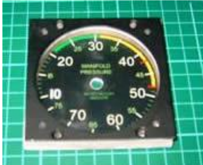
Figure 3-39. An assembled face plate for a flight instrument. Photo used with permission from Jan Verley. 34
