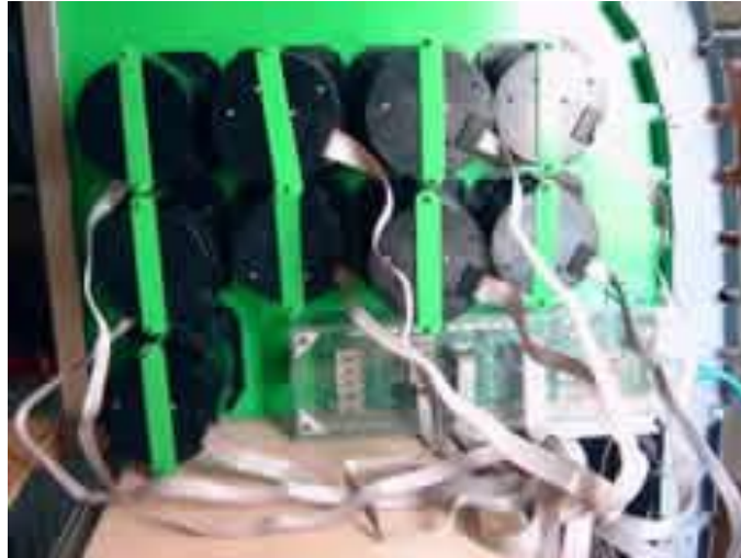
Figure 3-13. Back view of aircraft panel with USB controlled gauges mounted. Photo used with permission from Jan Verley. 9
