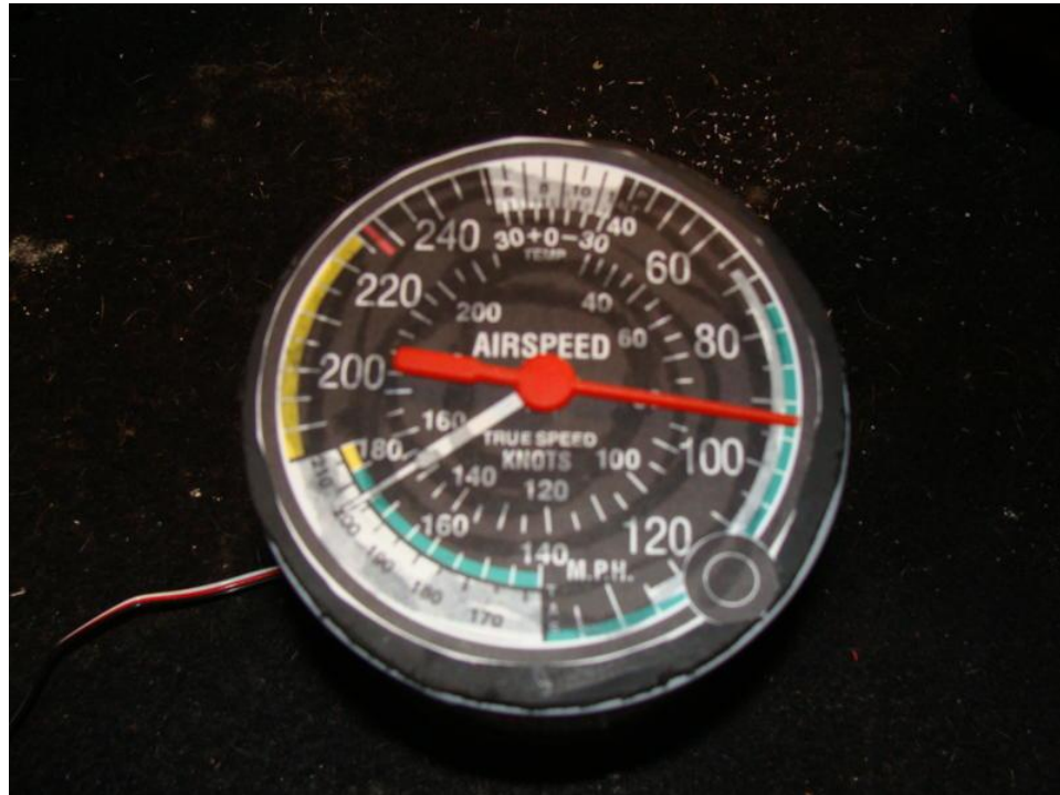
Figure 3-43. Assembled flight instrument with face plate and needle. Photo by Joseph Munera
