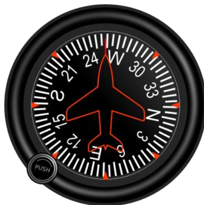
Figure 3-31. Face plate of the heading indicator. Used with permission under the GNU Free Documentation License 27
