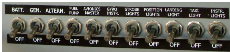
Figure 2-13: Switches of the GoBosh cockpit. Photo by Robert Gysi.
