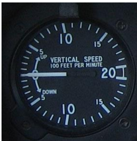
Figure 3-22. Face plate of the vertical speed indicator. This work has been released into the public domain by the copyright holder, Benet Allen. 16
