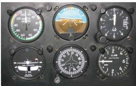
Figure 3-11. Closeup of the standard “Six-Pack” – Wikipedia used with permission under the GNU License 8
