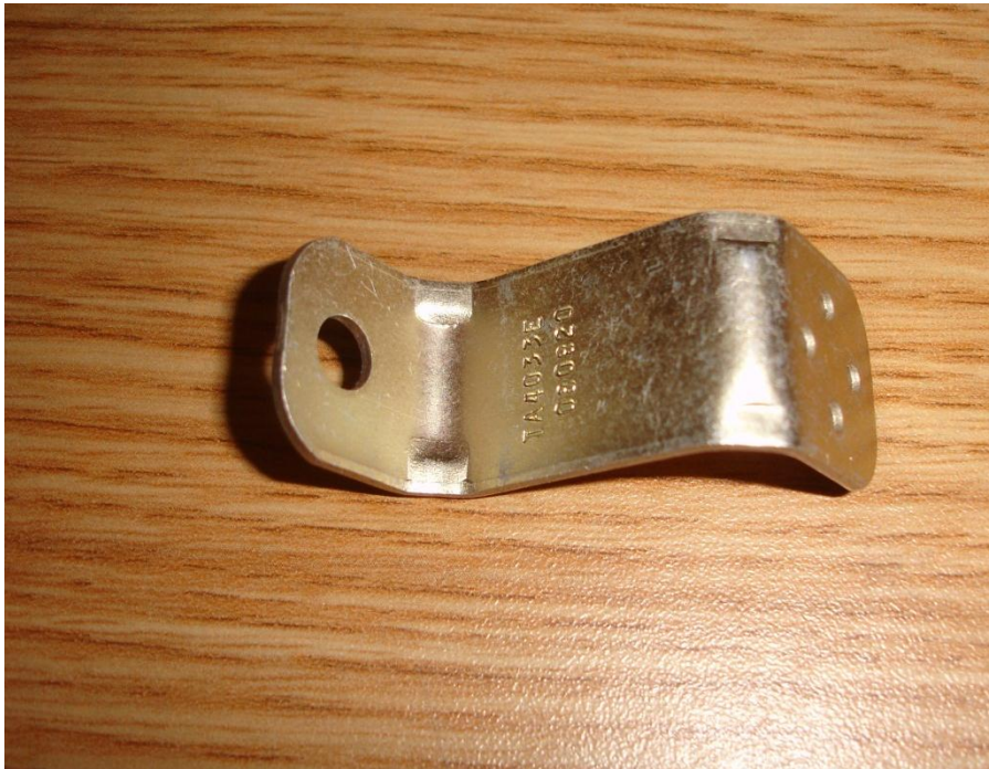
Figure 3-48. Angle bracket for connecting to flight control wire. The connecting screw to the potentiometer would be placed on the solid surface appromatel where the engraved text is located. Photo by Robert Gysi
