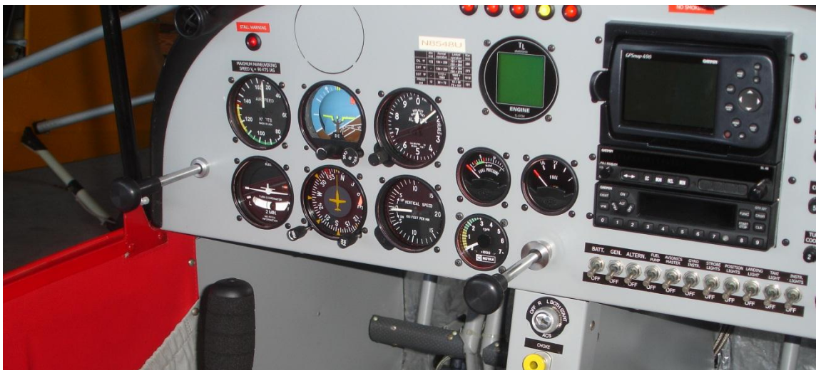
Figure 3-51. Throttle location (black knob pulled out of instrument panel). Photo by Robert Gysi
