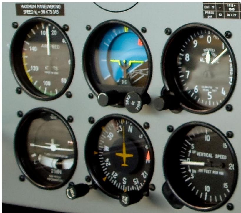
Figure 2-10: This is the standard six-pack of gauges in the GoBosh. Photo by Robert Gysi.
