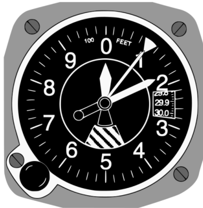
Figure 3-16. Altimeter Face plate, dials, and barometric pressure adjustment knob. This image has been released into the public domain by its author, Bsayusd at the Wikipedia project. 10
