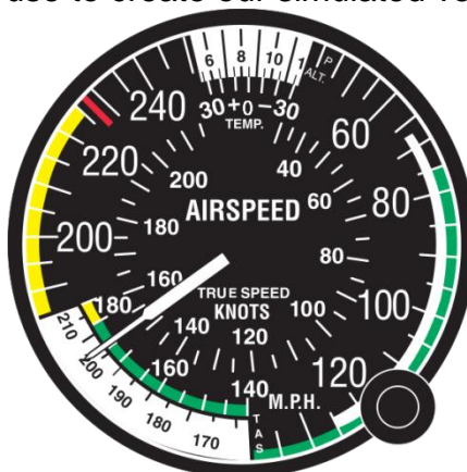
Figure 3-19. Airspeed Indicator Faceplate - Wikipedia. Used with permission under the GNU Free Documentation License 13
