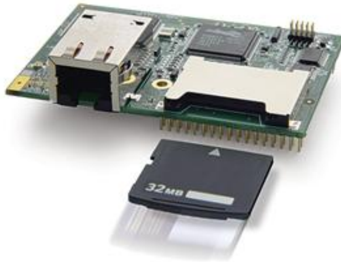
Figure 5.24: Figure shows the diagram of RabbitCore with removable memory card and Ethernet connection and on-board microprocessors. Reprinted with permission from Z-World Inc., see the Appendix Section A.3.
