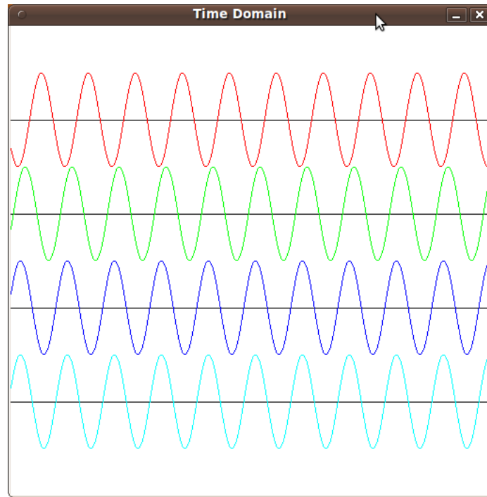
Figure 6.1: An example of the input signals of the simulated hydrophones digitally sampled.
