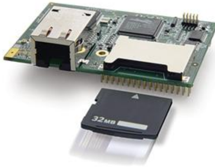
Figure 5.23: Figure shows the diagram of RabbitCore with removable memory card and Ethernet connection and on-board microprocessors. Reprinted with permission from Z-World Inc., see the Appendix Section A.3.
