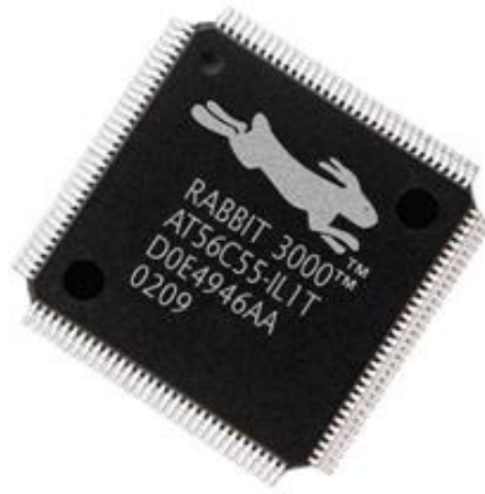
Figure 5.24: Figure shows the on-board microprocessor embedded on the RabbitCore. Reprinted with permission from Z-World Inc., see the Appendix Section A.3.
