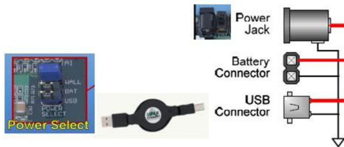
Figure 5.8: Set the jumper to wall and connect the power cord to power the board. Reprinted with permission from Digilent Inc., see the Appendix Section A.2.
