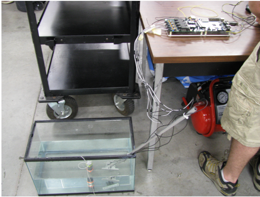
Figure 8.8: The overall system with hydrophones and pinger attach to the device
