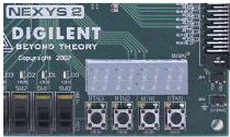
Figure 5.10: The seven segment display with 4 pushbuttons. Reprinted with permission from Digilent Inc., see the Appendix Section A.2.
