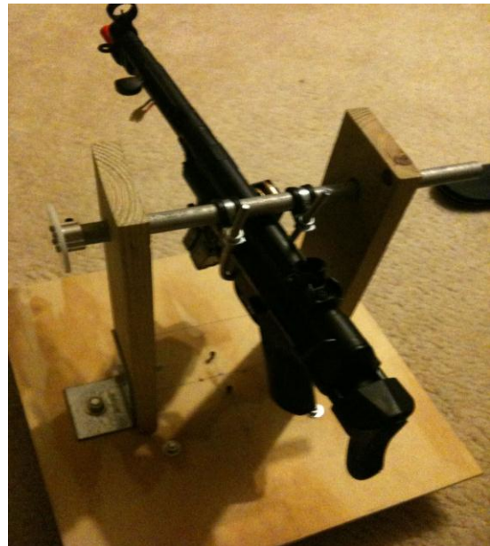
Fig. 1. Airsoft gun mounted on to our rotating base. The rod going through the top allows the gun to also tilt upward and downward.
