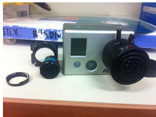
Figure 14. GoPro's Hero with original lens replaced with a non-fish eye lens.
