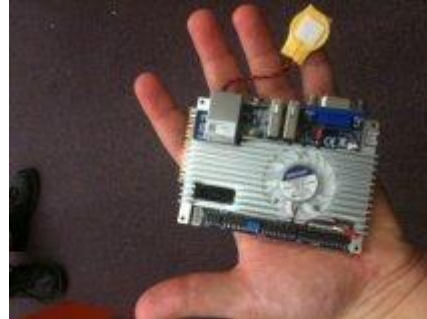
Figure 10. VIA Windows board form factor: Pico-ITX
