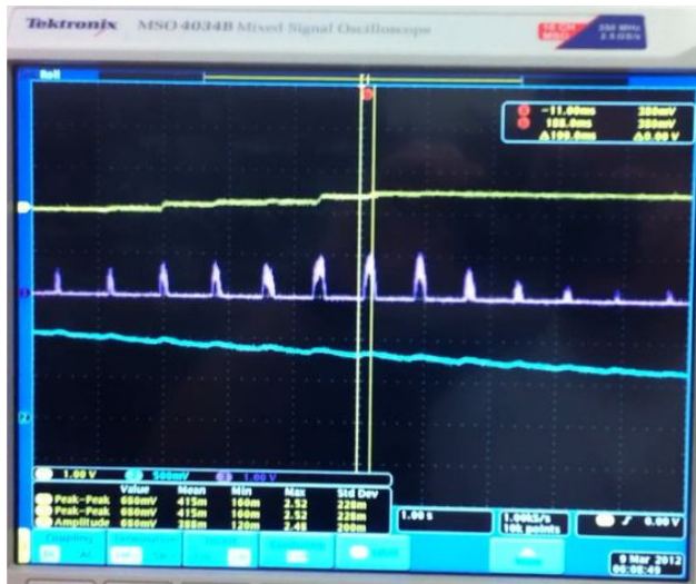
Fig. 4. The yellow line (top) represents the peak detection; the purple line (middle) represents the oscillation/pulse signal; the blue line (bottom) represents the cuff pressure decreasing.
