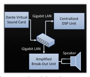
unit we are proposing. It will intercept eight to sixteen channels from ethernet, apply filtering and dynamics processing, and reintroduce the processed audio into the network. The device depicted at the bottom of the graphic is a break-out box
