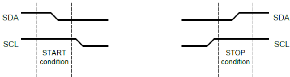
Figure 54:I2C Start and Stop Conditions
