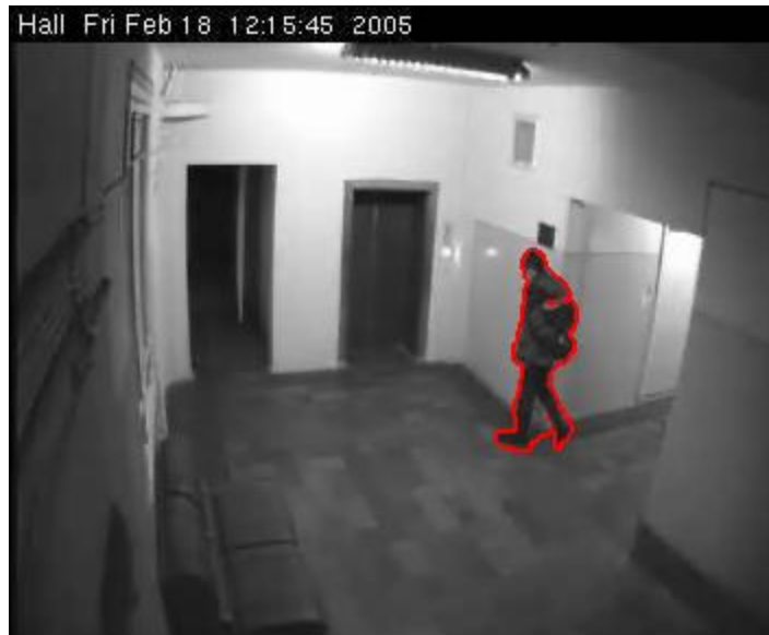
Figure 4.5.3.2-1: AForge motion border highlighting processing algorithm
