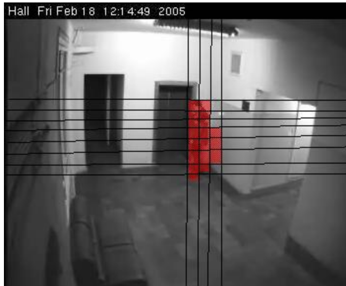
Figure 4.5.3.2-2: AForge grid motion area processing algorithm
