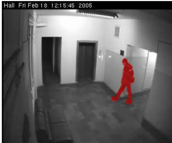
Figure 4.5.3.1-3: AForge simple background modeling motion detector algorithm
