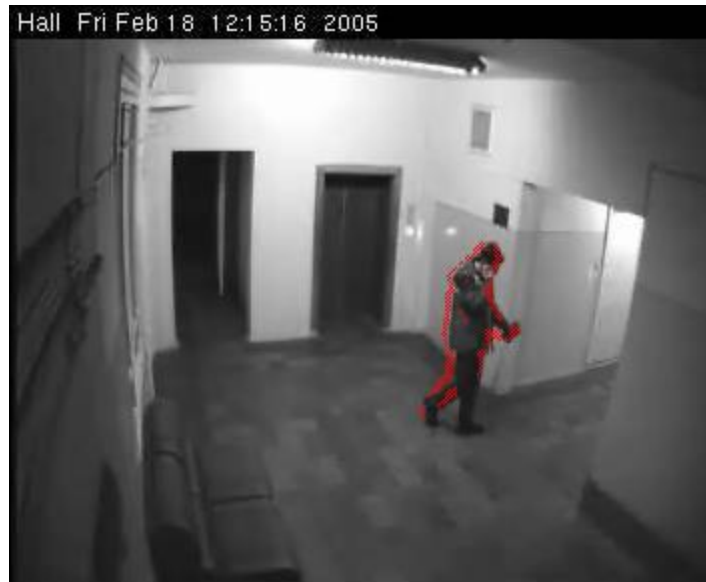
Figure 4.5.3.1-2: AForge two frames difference motion detector algorithm
