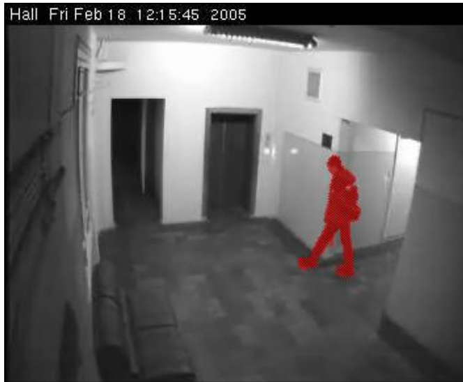
Figure 4.5.3.1-3: AForge simple background modeling motion detector algorithm
