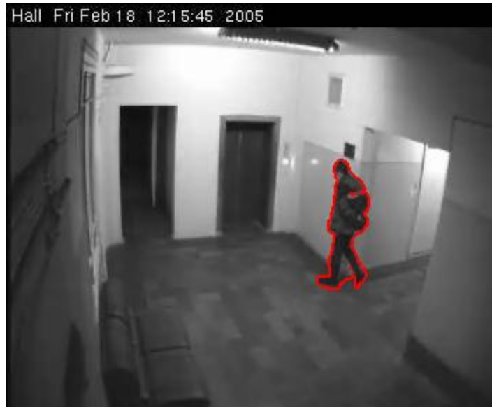
Figure 4.5.3.2-1: AForge motion border highlighting processing algorithm
