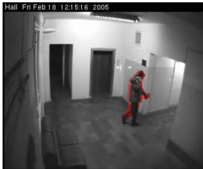
Figure 4.5.3.1-2: AForge two frames difference motion detector algorithm
