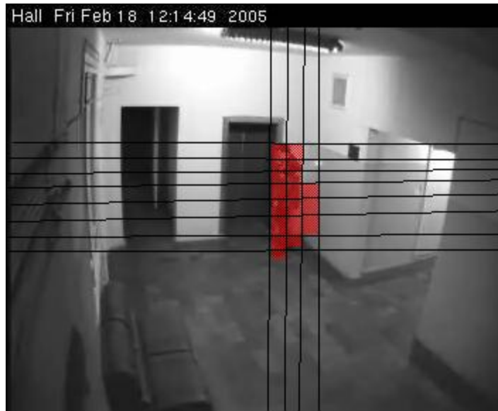
Figure 4.5.3.2-2: AForge grid motion area processing algorithm
