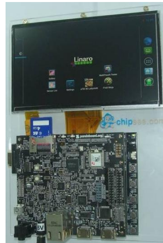
Figure 2: Pandaboard ES with expansion board
