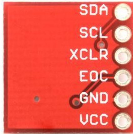
Figure 4.1.5.1: BMP085 Pin Connection with IOIO Reprinted with permission from Sparkfun.com[3]
