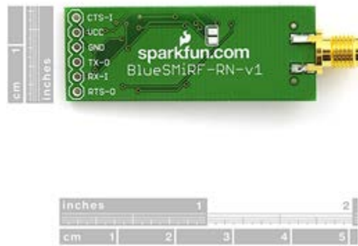
Figure 16: BlueSMiRF RP-SMA pin layout
