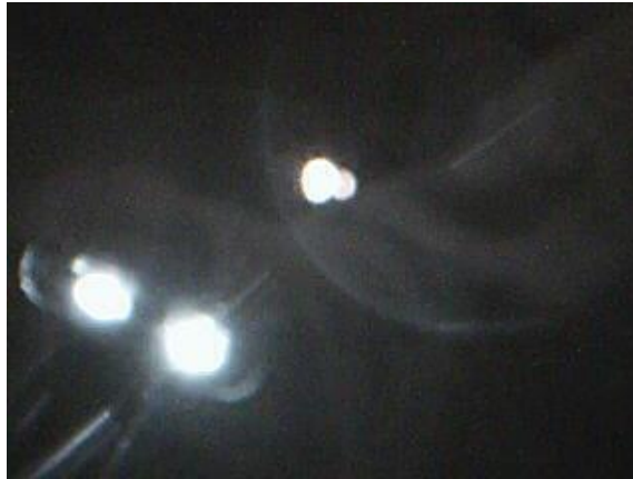
Figure 7: Infrared LEDs seen with the IR filter removed and the visible light filter
