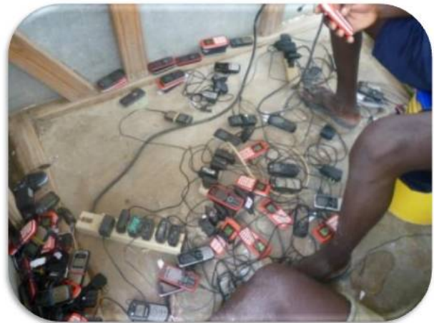
Fig. 1. Previous system used for charging in mobile devices from a pump’s power system, located in a remote village in Haiti.
