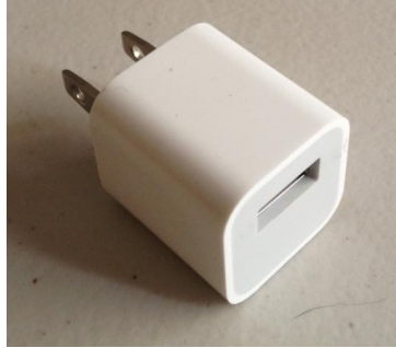
Figure 6 Apple Charging Unit
