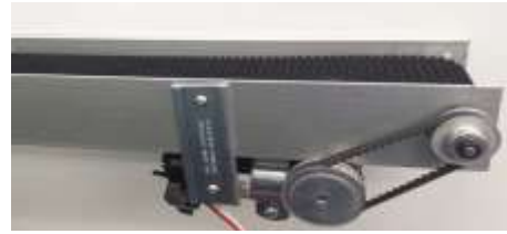
Fig.11. Puck-Return Gear Motor Drive
