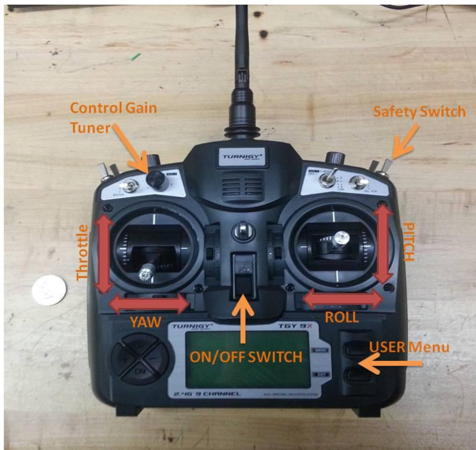
Figure 60: Turnigy Controller Unit Diagram
