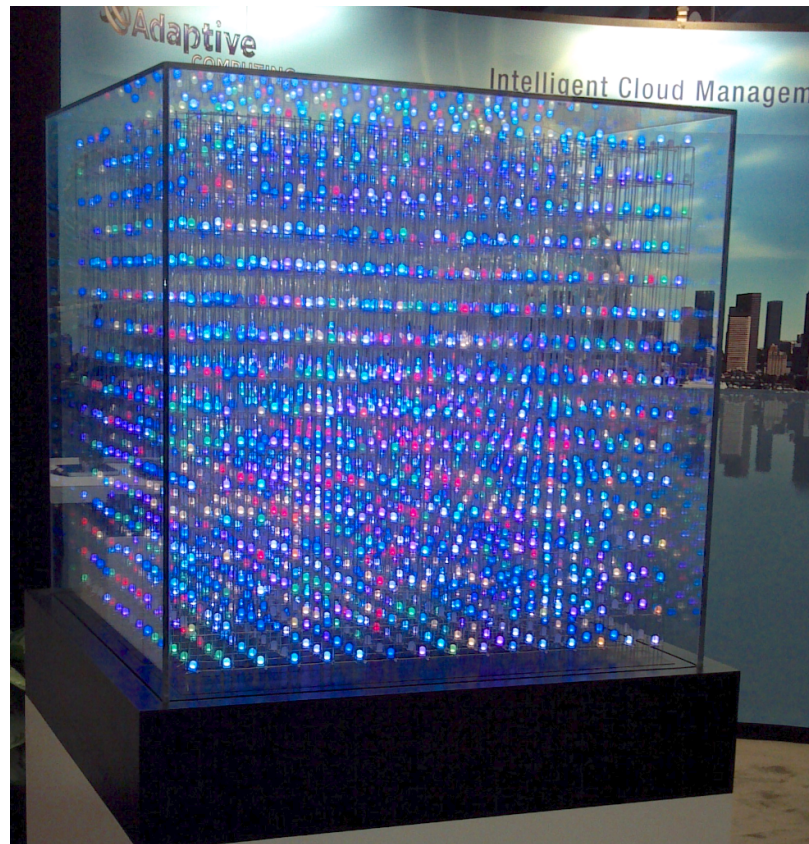
Figure 3.3: All Spark 16x16x16 3D RGB LED Cube Printed with Permission, Courtesy of AllSparkCube.com [2]
