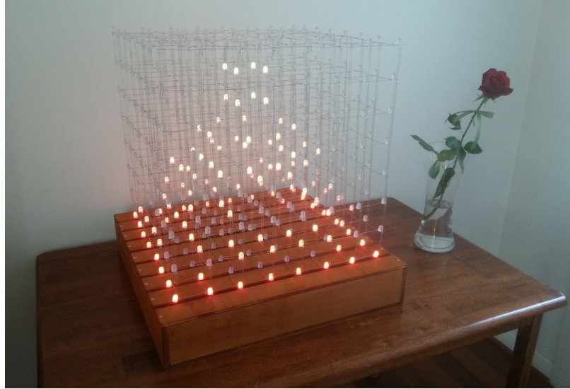
Figure 3.6: HNTE 8x8x8 3D RGB LED Cube Printed with Permission, Courtesy of HowNotToEngineer.com [4]
