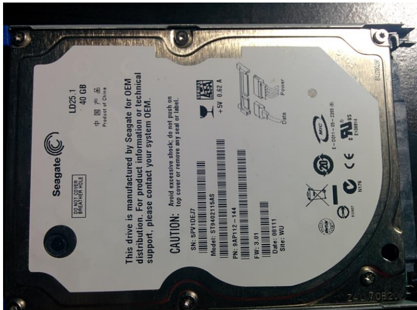
Figure 3 – 5: A Seagate internal laptop (2.5" form factor) hard drive with SATA interface.
