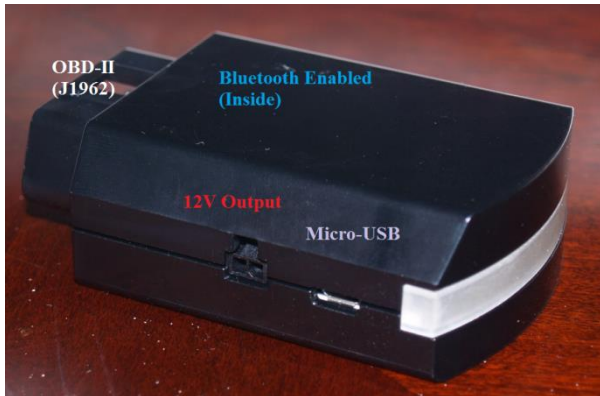
Figure 2: Vehicle Interface module and its features.
