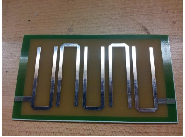
Figure 3. 978MHz Hairpin Filter on PCB
