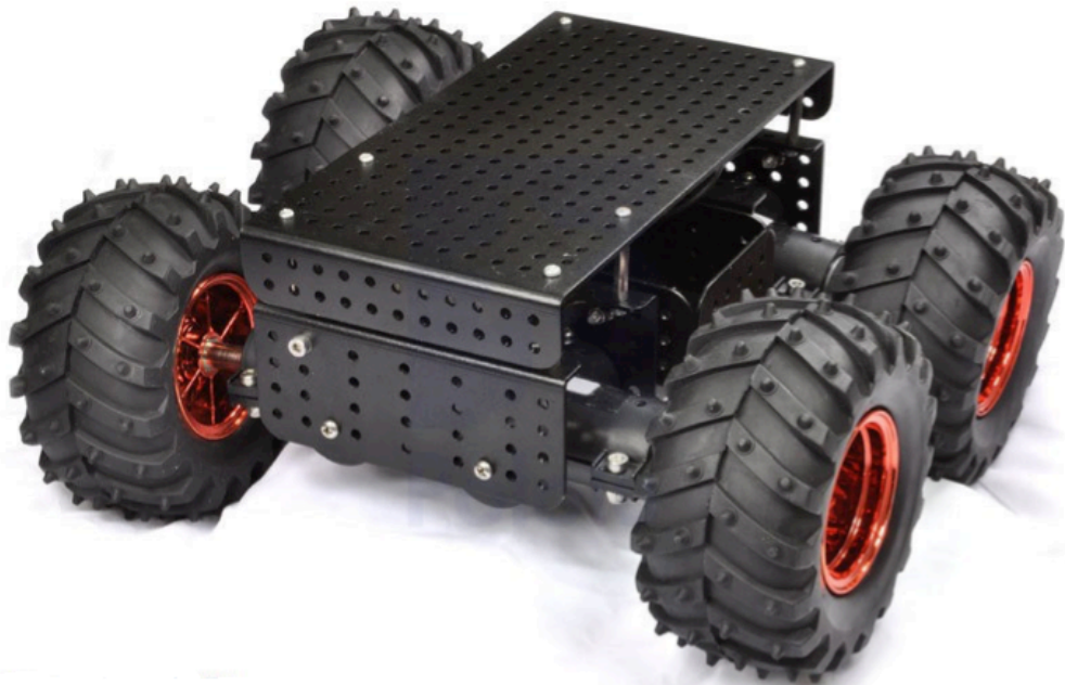
Figure 5.1.10.A - Dagu Wild Thumper 4WD All-Terrain Chassis Pending permission from Pololu
