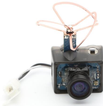
(Figure 3.32 shows the SPMVA1100 camera module) [26]
