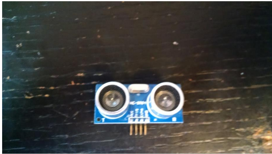
(Figure 3.12 shows the SR-04 sensor)
