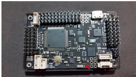
Fig.4. ArduPilot Module (APM) 2.8
