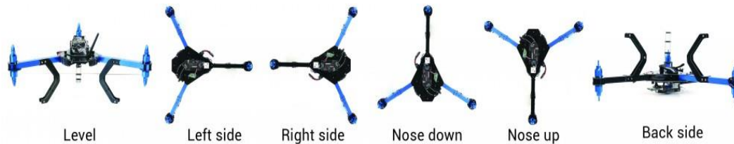
Figure 42: Accelerometer Calibration Positions (copter) (Permission Pending)
