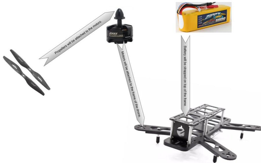
Figure 57: Final Look of 3K-QAV250, Motors, Propellers & Battery
