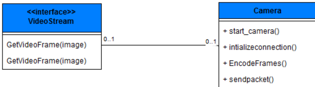
Figure 49: Class Diagram of the camera streams.
