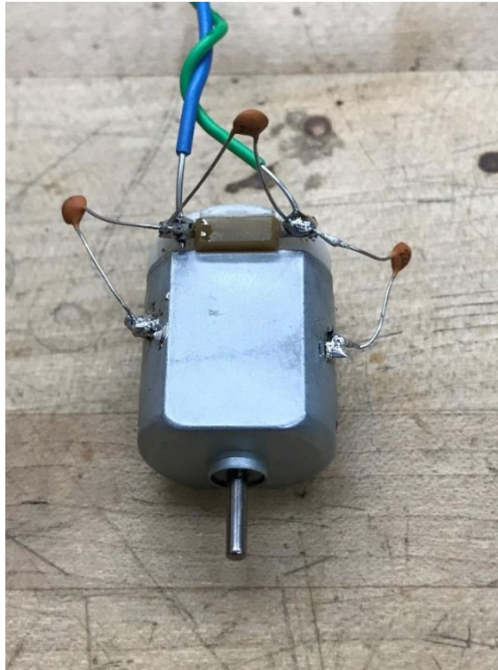
Figure 10.2 – Brushed DC motor with Capacitor Noise Filters
