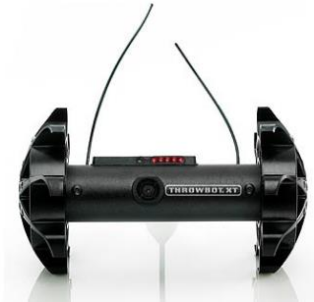
Figure 3-1: Throwbot XT vehicle made by ReconRobotics [1]
