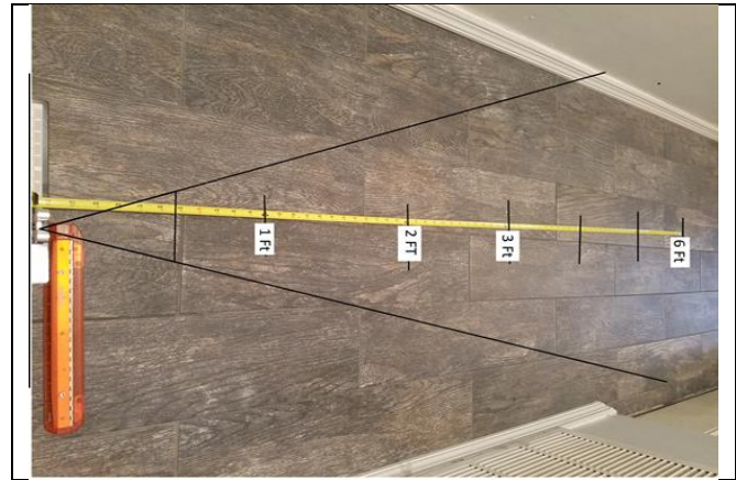
Figure 3: Example of viewing angle of ultrasonic sensor
