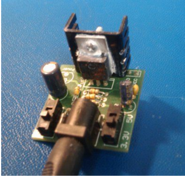
Figure 20: Voltage regulator with a heat sink [89]
