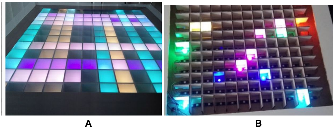
Figure 2: A) The finished product of the LED coffee table. B) The LED housing grid.
