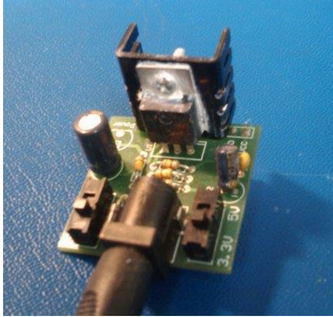
Figure 20: Voltage regulator with a heat sink [89]
