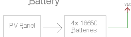
Figure 3.4.i Rough Draft Power System Schematic
