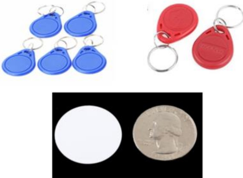
Figure 36: High Frequency RFID (top left), Low Frequency RFID (top right) NFC Tag (bottom)
