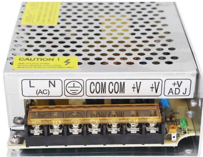
Figure 15. Aiposen S-120-12 Connections. Permission requested from Amazon Inc [18]
