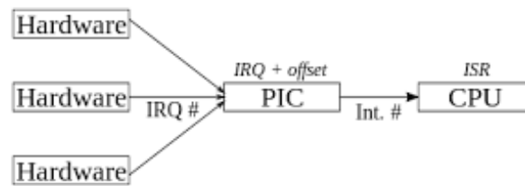
Figure 12: Hardware Interrupt Flow Diagram (Public Domain)
