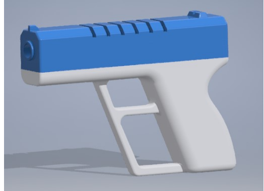
Fig. 1. 3D model of laser tag “gun” housing created in Autodesk Inventor
