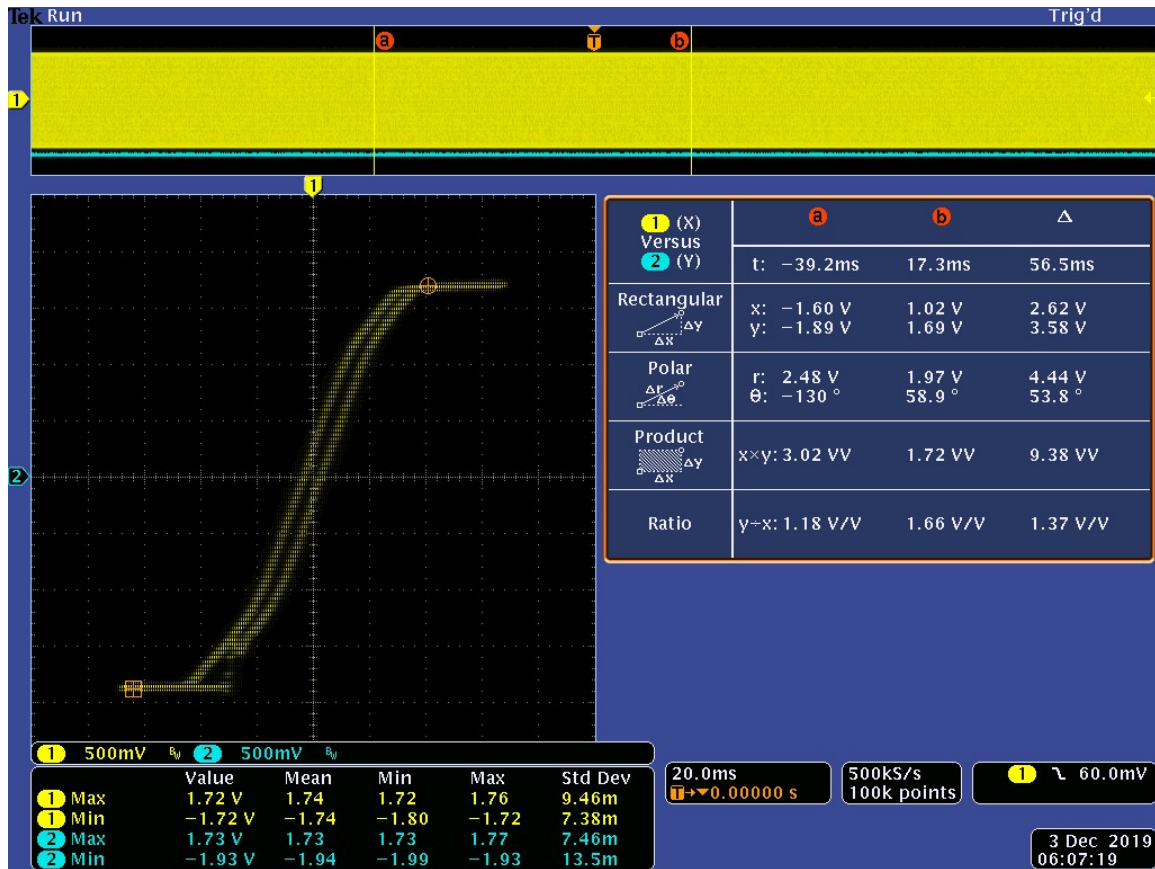
Figure 8.5: TL084-based neuron response at 20 kHz
