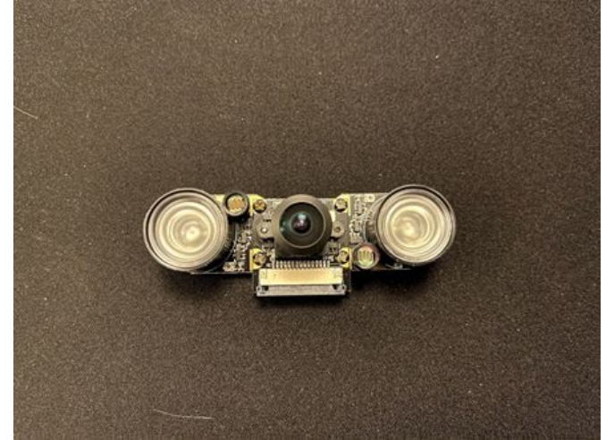
RPi Camera with attached infrared LEDs
