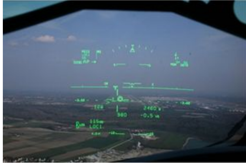
View of a HUD from inside an airplane from the perspective of a pilot
