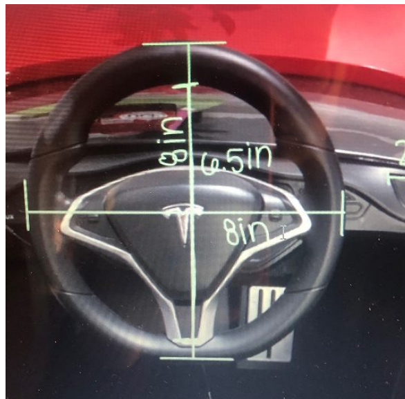
Figure 54. Dimensions of Steering Wheel
