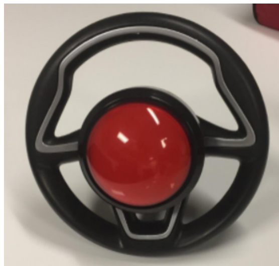
Figure 57. LED Arcade Button inside Steering Wheel
