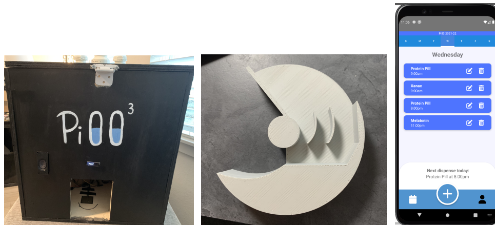
Figure 50: (a) Chassis of Pill 3 , (b) Sorting Disk, (c) Mobile App
