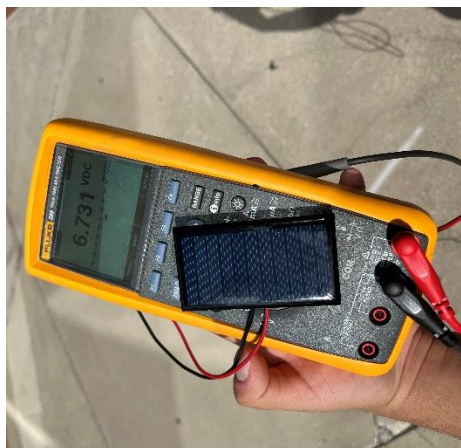
Figure 23 - Solar Panel voltage testing
